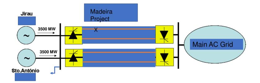
For a pole outage, apply the overload in the other 3 Poles, so as to keep the same Pdc level.
